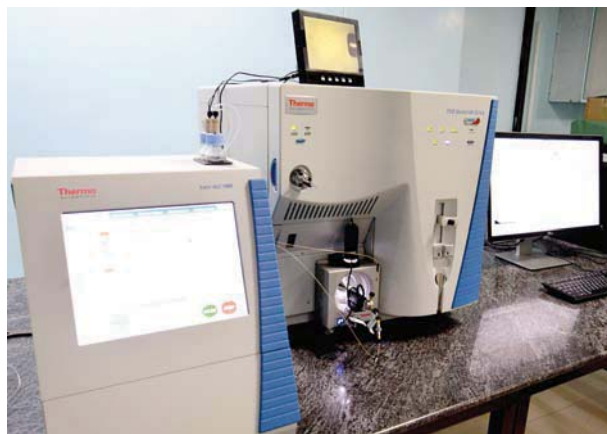
TSQ Quantum Ultra™ triple quadrupole mass spectrometer for high-throughput and accurate quantitation of proteins
